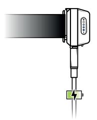
During the charging process, the LED battery capacity indicator (05) flashes blue. After approx. 2 hours the battery is fully charged and all 4 LEDs of the LED battery capacity indicator (05) light up constantly blue. Disconnect the headlamp from the USB charging source and properly close the rubber cover (06a) to ensure splash protection.
