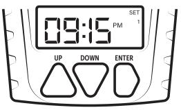
After entering the minutes, press the ENTER button (09) to set the **spreading duration** (second digits flash). Use the UP (07) and DOWN (08) buttons to select a spreading duration of **1-30 seconds**:
