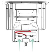
Carefully remove the battery box (11) from the battery compartment (10) without tearing off the cable connection.
