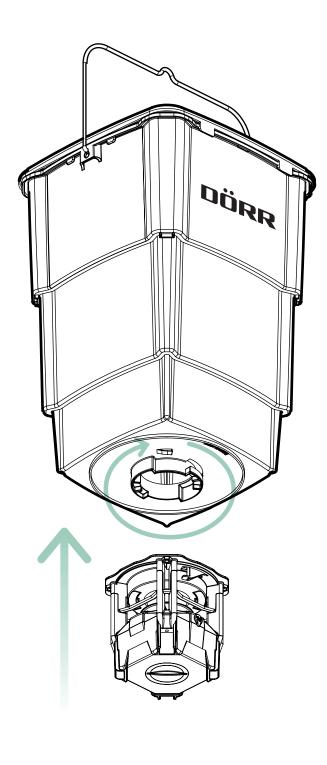
To remove the feed container, pull the two release clips (13) down and turn the feed to the left.
