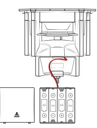
Slide the battery compartment cover (11a) back onto the battery box (11). Place the battery box (11) with the cable connection back into the battery compartment (10) and press the battery box back down into the holder.
