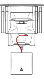
Slide open the battery compartment cover (11a) according to the marking in the direction of the arrow. Equip the battery box with **4 pieces Mignon batteries AA LR6 1.5V or or equivalent rechargeable AA batteries** (not included). **When inserting the batteries, pay attention to the correct polarity +/-** (markings inside the battery box).
