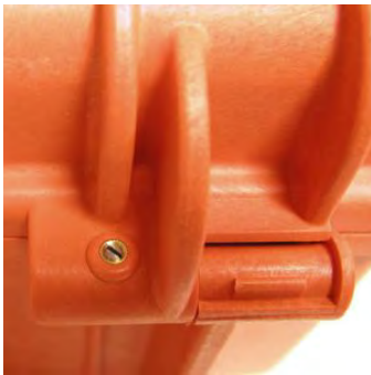
LID CAN BE SET TO SLIDE-OFF By releasing the back screw, lid becomes set to slide-off when opened at 70°
