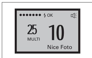
Example: You wish to flash 15x during 1 exposure. Set the number of 15 flashes. In order to achieve a short exposure time, set the shortest possible flash frequency of 10 flashes per second.
