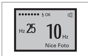
1. Frequency of Flashes: Press the MENU button repeatedly until the LCD shows 2 figures and Hz. This is the number of flashes fired during a picture (small figures on left-hand side) and the frequency - time between the flashes (figures on right hand side). Use the UP and DOWN keys to select a flash frequency between 1 and 10. 1 corresponds to approx. 1 flash/s, 2 approx. 2 flashes/s ..... 10 equals approx. 10 flashes/s.
