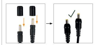
Open the rubber cover OUT (06a) on the solar panel. Then plug the connection cable (09) into the output socket OUT (06) of your solar panel and the other end into the "Connection external battery" of your SnapShot 4G Camera. Turn on the camera – the solar panel will recognise when a consuming device is connected and starts the power supply.
