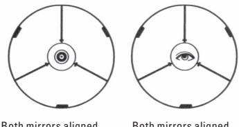
Both mirrors aligned with collimating cap in
