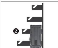
Hang the 4 motor drives A, B, C, D (1) with the guide slots (1a) into the ceiling/wall mount (3). Connect the cables of the motor drives to the 4 sockets (5a) at the control unit.
